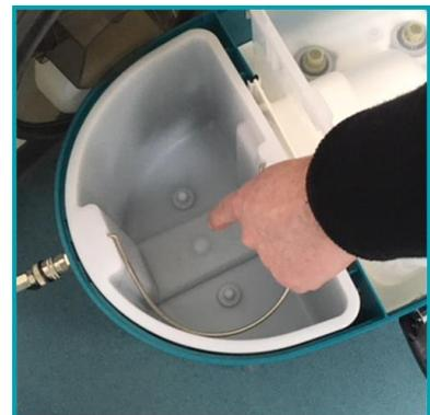
After a few passes, check the waste tank to see that no foam is present. Add extra defoamer if necessary.
