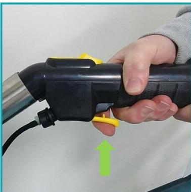
Press and hold the solution trigger to apply the cleaning solution, whilst pulling the wand or tool slowly backwards to clean the carpet or upholstery.
