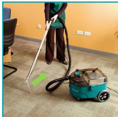
Move the wand backwards and repeat, slightly overlapping the previous pass. Do not clean any area more than twice, or overwetting could result in carpets and upholstery shrinking.
