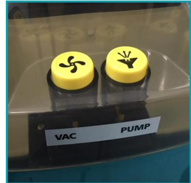
Switch on the pump spray and/or vacuum.
