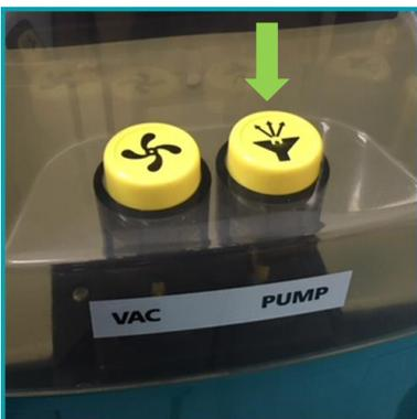
Turn on the PUMP switch. This will pump out any remaining solution.
