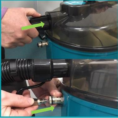
Connect the vacuum hose onto the vacuum hose inlet and the high pressure spray hose onto the solution outlet.
