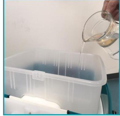
Fill the solution tank with mixed water and approved cleaning chemical according to the chemical manufacturer's instructions.
