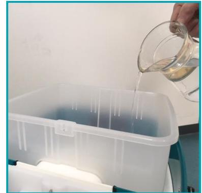
Add approx.  $\frac{1}{2}$  litre of clean water to solution tank to flush out the tank and pump.
