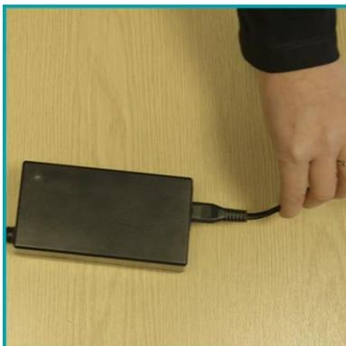
After every use check the battery cable for any wear or damage, check the dust bag and if full replace. Check the battery charge status and charge if required.
