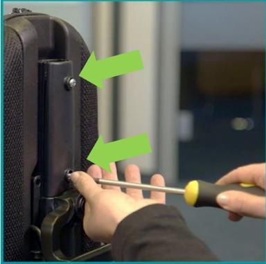
Remove the handle bracket by removing the two screws.
