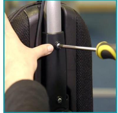
Place the handle bracket back into position and secure the two screws.
