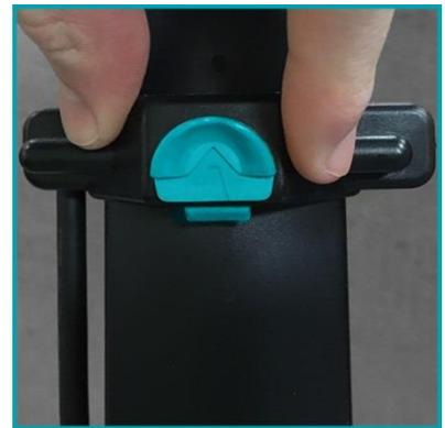
Hold the latch against the reverse side of the handle duct. Note latch orientation.
