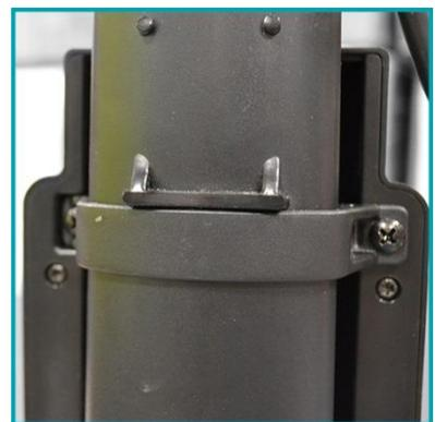
Please note that the battery clamp is currently positioned beneath the lug on the handle duct.
