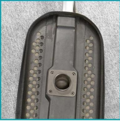
Lay the vacuum on its back and fit the bag compartment (1) onto the machine then replace the rubber gasket (2) so that the screw holes are aligned.
