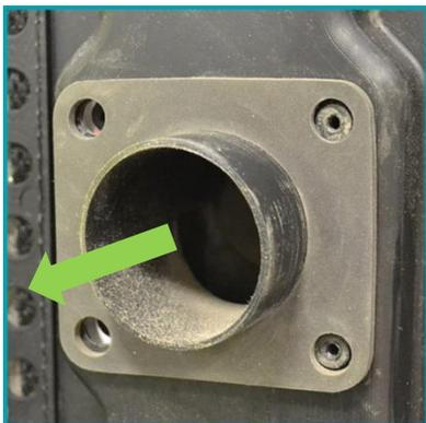
Remove the rubber gasket.
