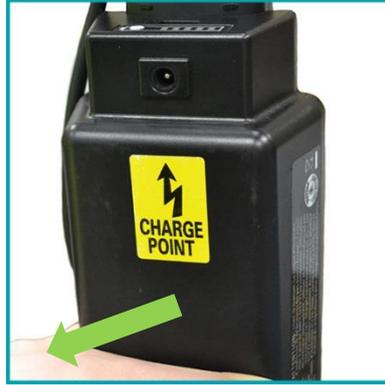
Remove the battery and battery clamp.
