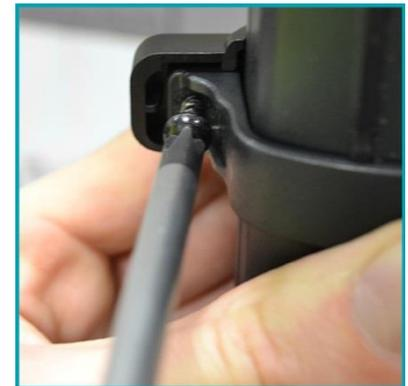
Secure the battery clamp to the latch by screwing the 2 screws.
