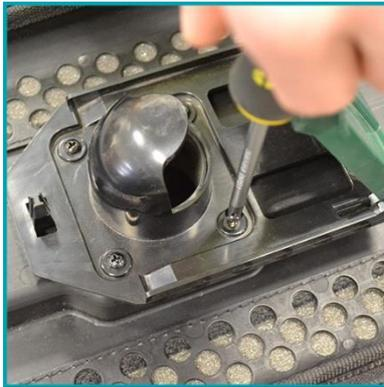
Lay the machine on the floor and undo the 4 screws surrounding the vacuum bag holder using a cross-head screwdriver.
